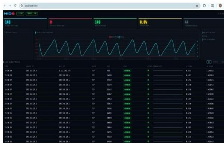
Figure 4: Real-time intrusion detection dashboard displaying network traffic monitoring and threat analysis.
