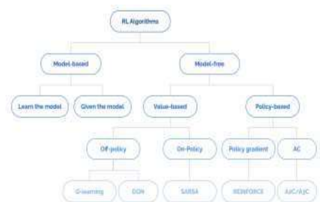
Fig. 4. A partial taxonomy of RL algorithms. DQN is Deep Q-Network, SARSA is state-action-reward-state-action algorithm, and AC is actor-critic.
