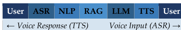
Figure 2. Voice-enabled multilingual legal interaction pipeline: ASR → NLP → RAG → LLM → TTS, supporting English and Telugu.
