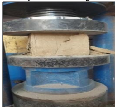
Fig 2 Experimental setup for unconfined compression testing of adobe specimens
