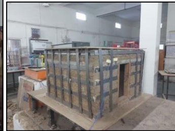
Fig 13 Model A2 On Shake Table
