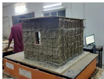
Fig 21 Model C1 On Shake Table
