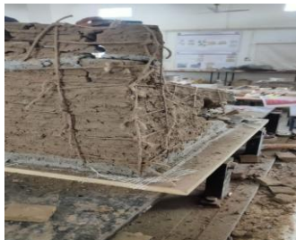
Fig 23 Collaose of Model C1
