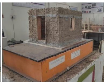
Fig 22 Model C2 On Shake Table
