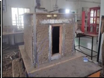
Fig 12 Model A1 On Shake Table
