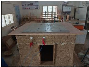
Fig 11 Model U1 On Shake Table
