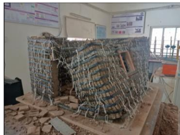
Fig 19 Collapse of Model B1
