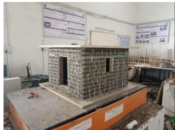
Fig 17 Model B1 On Shake Table
