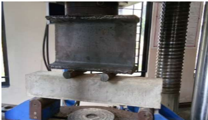
Figure 1. Four-point Bending Test on universal Testing Machine
