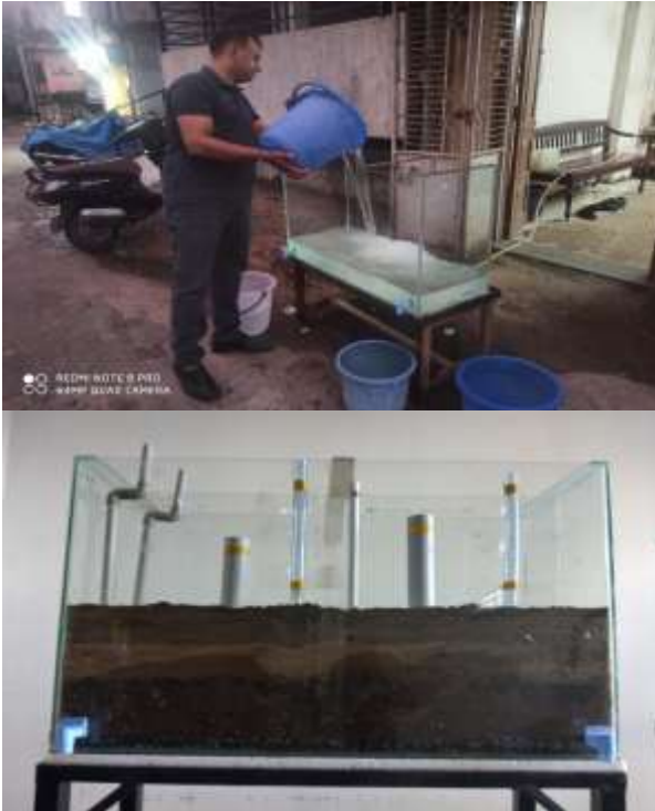
Figure 1: Checking Water tightness of Experimental Model and Final lab Experimental Model
