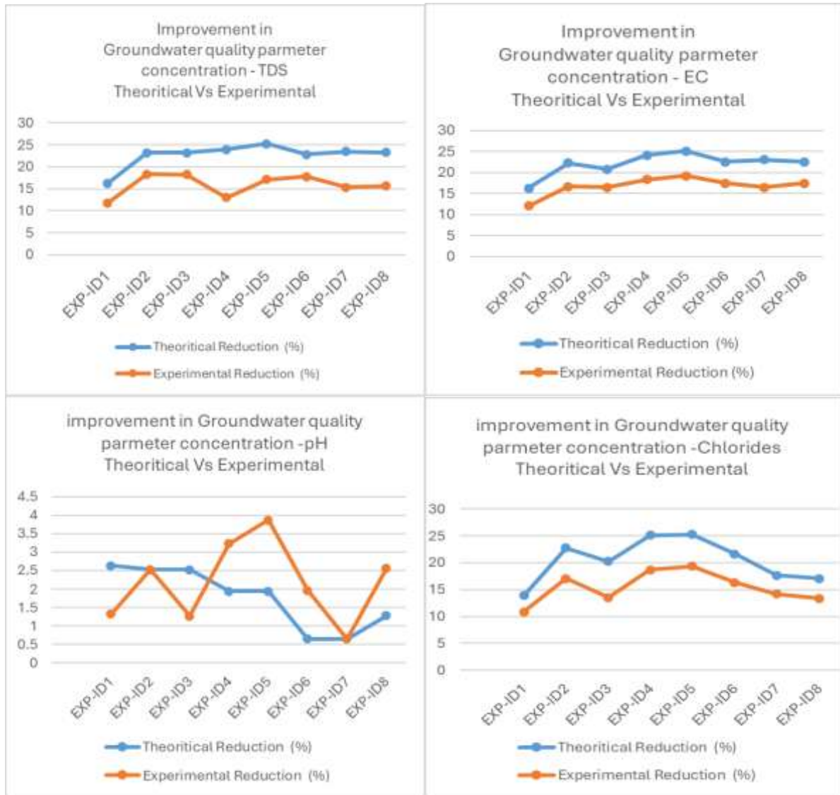
Figure 2: Comparative Scenario of Percentage reduction in Quality parameters by Theoretical vs Experimental methods
