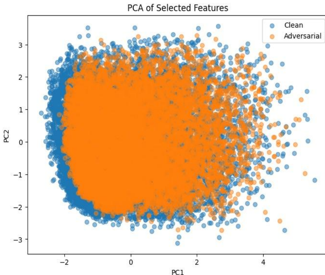
Figure 5: PCA-based visualization of clean and adversarial samples in reduced feature space, illustrating their distribution and partial separability.
