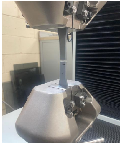
Figure 2: Tensile test setup for a Type I specimen according to ASTM D638-22 using a Shimadzu® AGS-X machine
