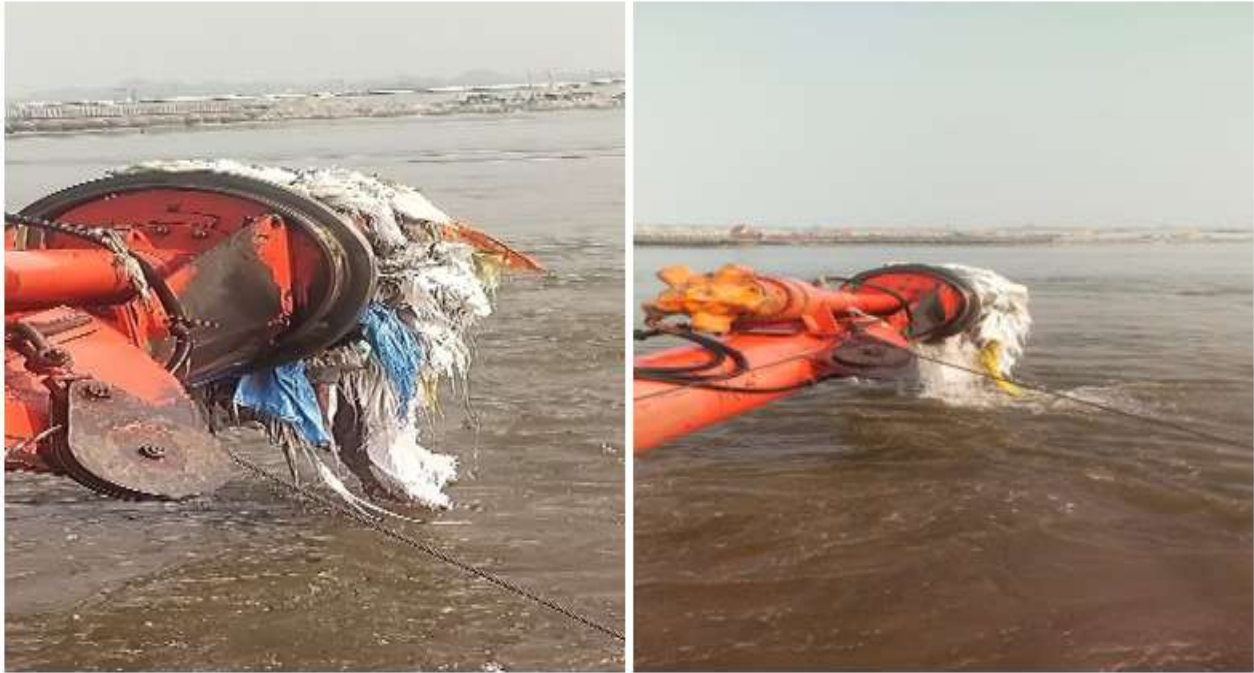
Figure 18: Materials Stuck in the Cutter and Suction
