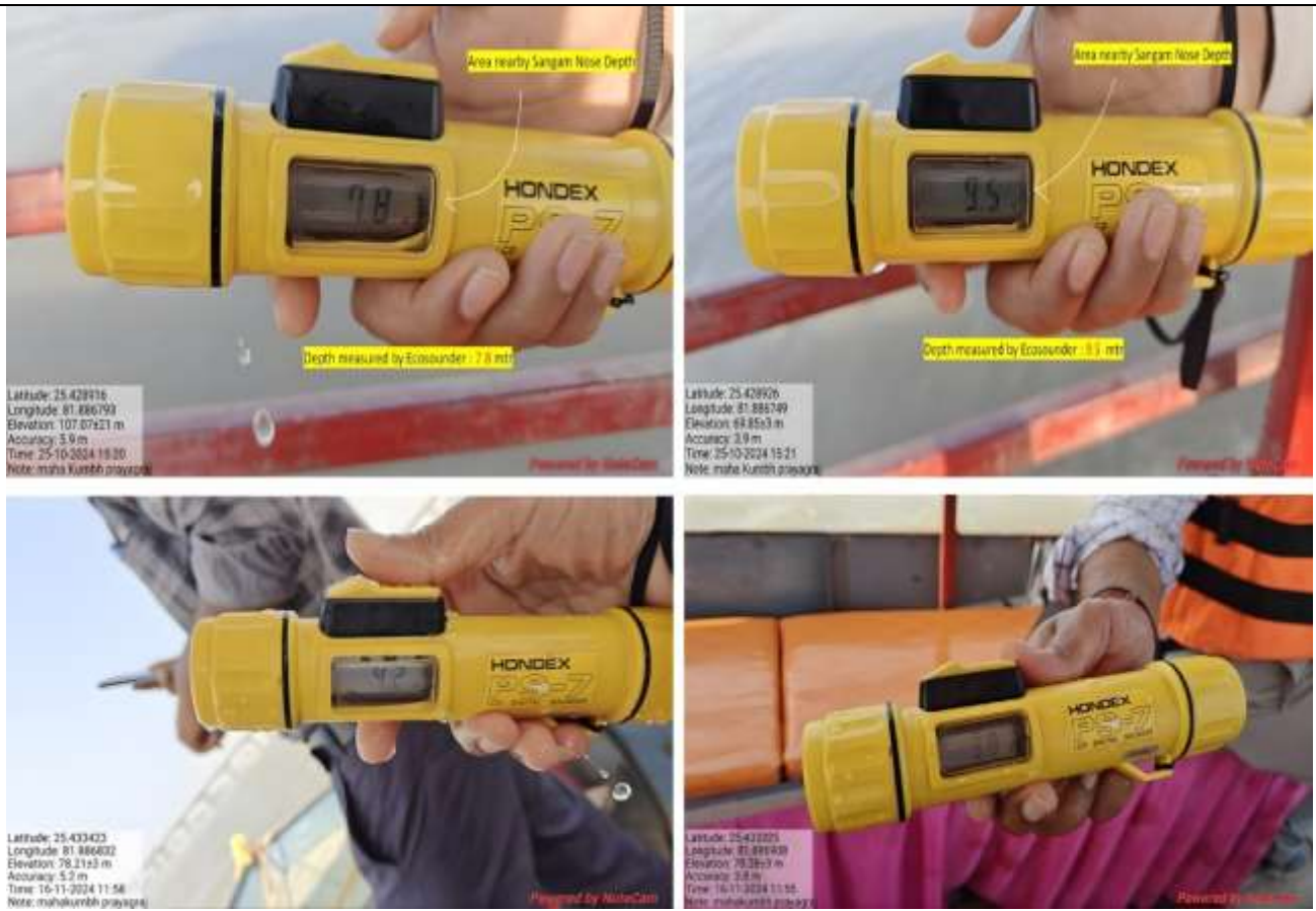
Figure 16: Depth Measured by Ecosounder at Different Locations in Ganga River Triveni Sangam showing detailed depth profiles obtained through acoustic surveying
