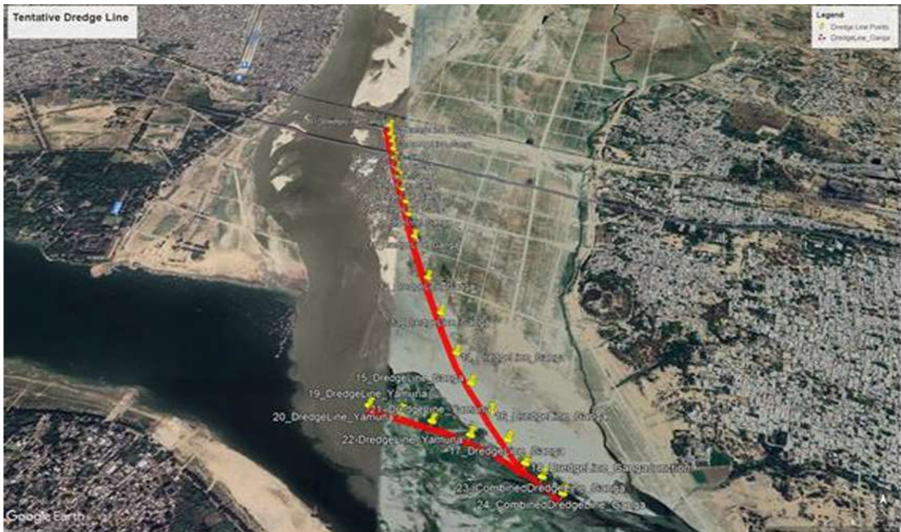
Figure 9: Tentative Dredging Path from Red Lines showing planned channel alignment and excavation zones
